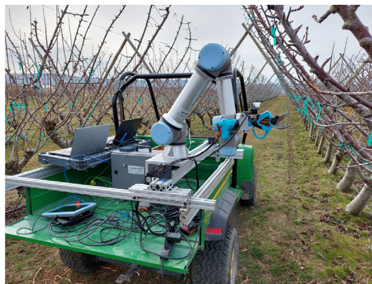
FIGURE 2 Our pruning robot during field trials. The pruning controller was trained entirely in simulation (You, Parayil, et al. 2022).
